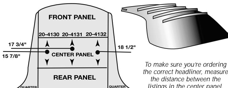
To make sure you're ordering the correct headliner, measure the distance between the listings in the center panel.
